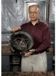
that looks like a cross between a lunar landing craft and a stop sign. Designed with a smooth airflow to fuel the fire and an upper rim that fits snugly with different-size pots, the stove requires 75 percent less wood than an open fire, and a wind collar makes for a steady flame. That means fewer risky trips outside the camp. And those who now pay for firewood, Gadgil estimates, could save as much as \$200 a year, which could be used instead for luxuries like new clothing and fresh meat.
